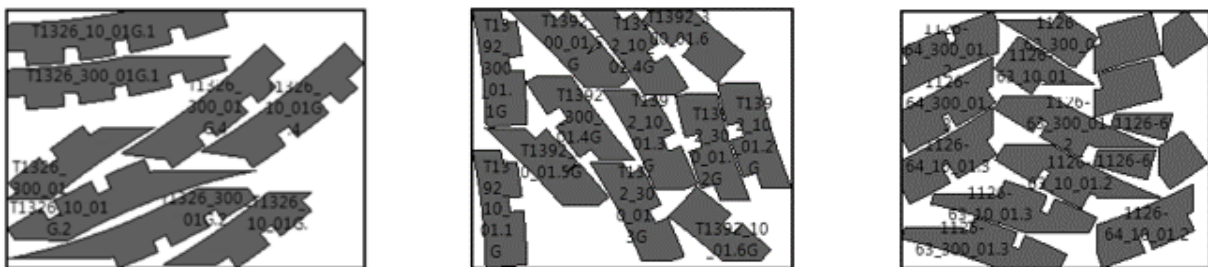
Figure 4: A traditional approach to a cutting plan. Material use from left to right is: 1.48m, 1.32m and 1.3m
