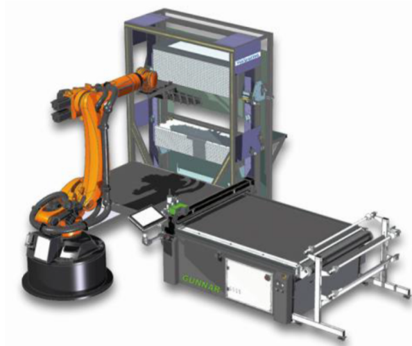
Figure 3: The sorting station has a robotic arm sorting composite plies on an automated vertically stacked tray system. A different kit is assembled on each tray, and trays move up and down to allow the robot to sort the plies between them
