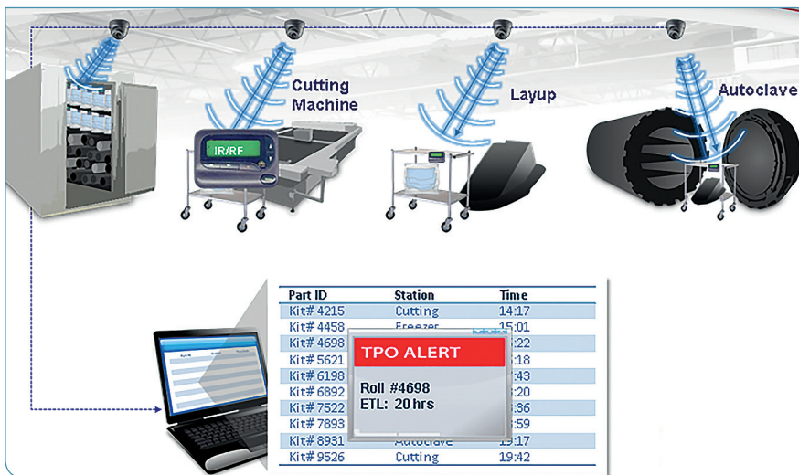
Fig. 1: Automatically tracking inventory and kits on the production floor to further increase productivity and reduce waste
